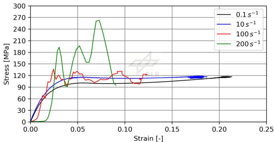
Figure 3: Dynamic stress-strain data of  $\pm 45^\circ$  tensile specimens for in-plane shear properties at different strain rates without damping materials.
