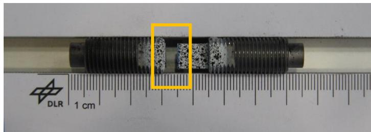
Figure 6: Failed transverse tension specimen after dynamic testing at a strain rate of  $0.1 \text{ s}^{-1}$ .
