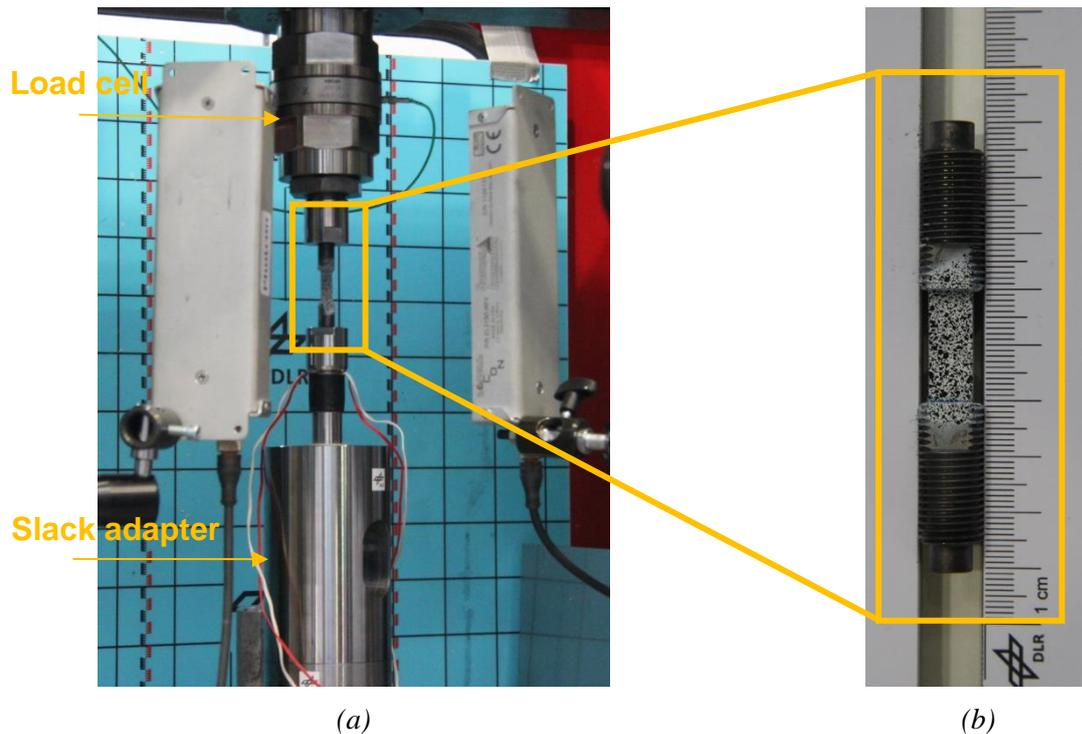
Figure 1: Dynamic testing set-up: (a) Test system with a test device and a test specimen, and (b) In-plane shear specimen.
