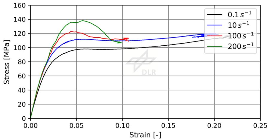
Figure 4: Dynamic stress-strain data of  $\pm 45^\circ$  tensile specimens for in-plane shear properties at different strain rates with damping materials.
