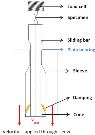
Figure 2: An illustration of a test device, slack adapter.
