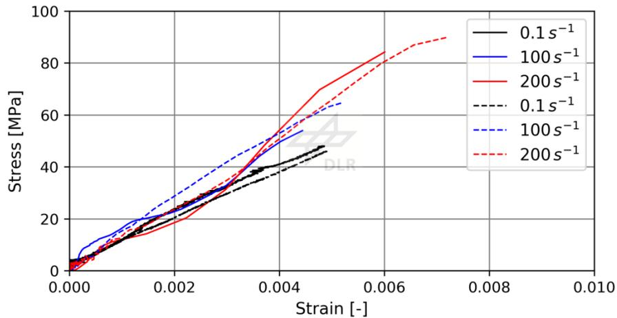
Figure 5: Dynamic stress-strain data of 90° tensile specimens for transverse tension properties at different strain rates without (solid lines '-'), and with damping materials (dot lines '--').
