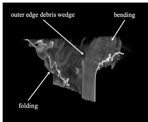
Figure 3: Micro-CT images of failure in CF-BA specimens.
