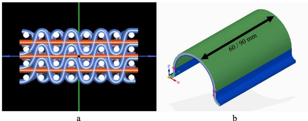
Figure 1: Diagrammatic representations of (a) layer-to-layer weave architecture (b) omega-shaped geometry
