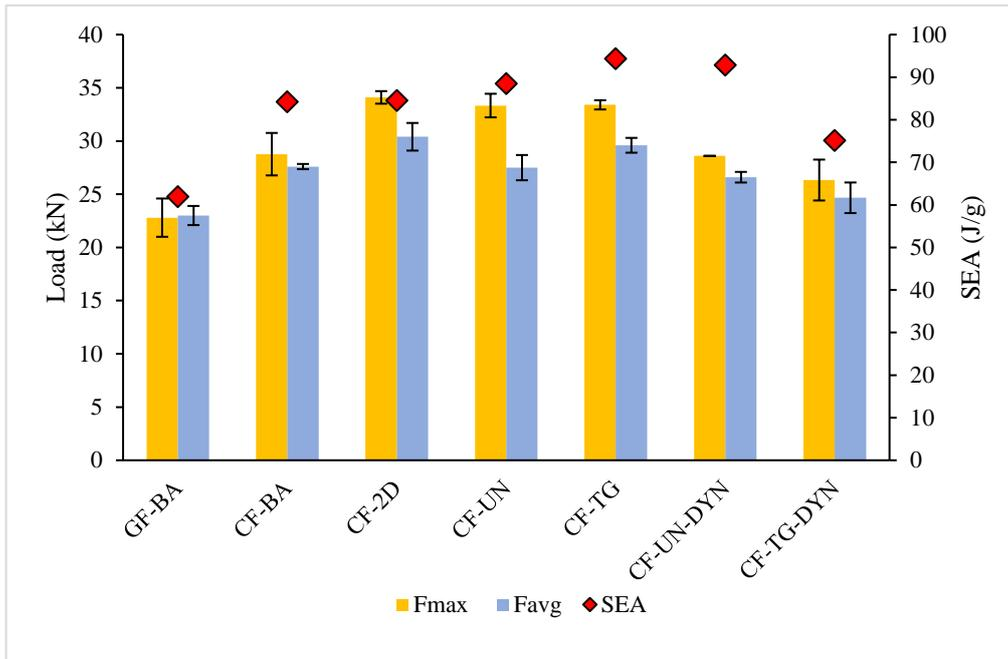
Figure 2: Crush results for all specimens tested.
