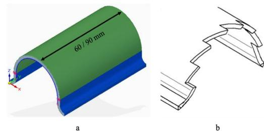
Figure 2: (a) Omega-shaped specimen (b) saw-tooth trigger
