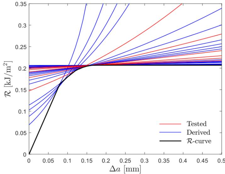
Figure 4: Numerical prediction of the  $R$ -curve (in black), and tested (in red) and derived (in blue)  $G_I(\Delta a)$  curves.
