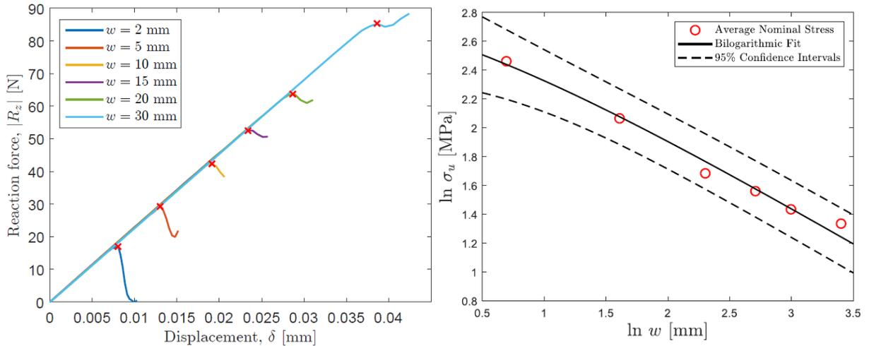
Figure 2: Numerical predictions of load-displacement for different virtual SENT specimen widths (left), and corresponding bilogarithmic size effect law of the peak loads,  $\sigma_u = \sigma_u(w)$  (right).
