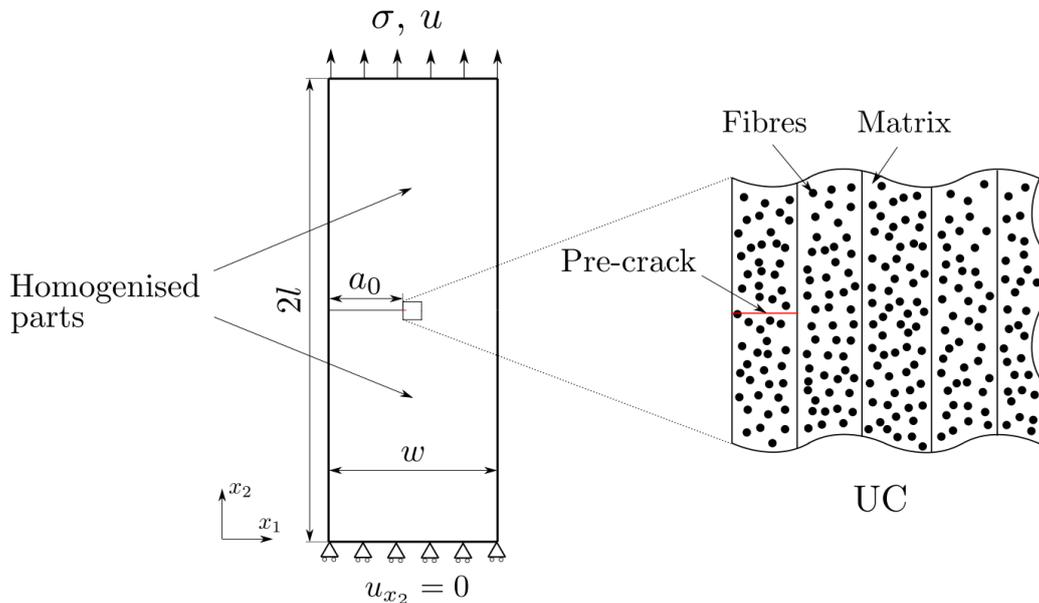
Figure 1: Schematic representation of the FE models and applied BCs.
