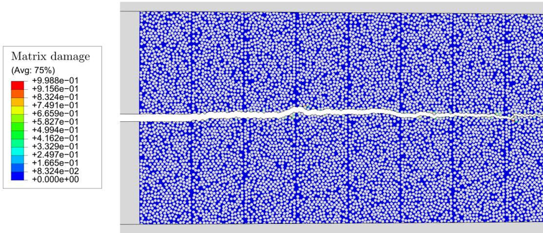
Figure 3: Contour plots of the matrix damage variable (Equation (3)) of a FE model having  $w = 10$  mm.
