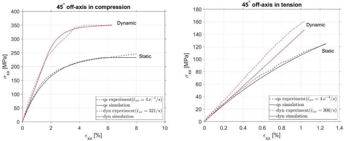
Figure 3: Quasi-static and dynamic axial stress-strain curves for the experiment and simulation of 45° off-axis in compression and tension [2,3]
