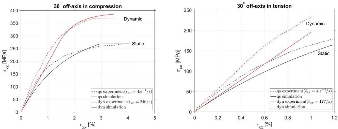
Figure 4: Quasi-static and dynamic axial stress-strain curves for the experiment and simulation of 30° off-axis in compression and tension [2,3]
