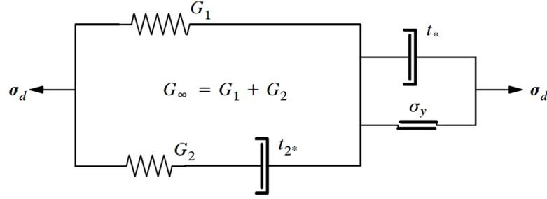
Figure 2: Rheological model for the in-elastic response of the matrix of the composite. It consists of a viscoelastic 3 parameter response combined with a viscoplastic deformation mechanism.
