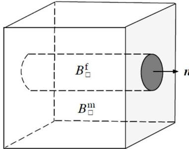
Figure 1 : Representative volume element of composite with volume  $V_{\square}$  with a fibre region  $B_{\square}^f \in B_{\square}$  (with the fibre orientation  $\mathbf{n}$ ) embedded in the polymer matrix  $B_{\square}^m \in B_{\square}$ . In the different regions it is assumed that the micro-stresses  $\boldsymbol{\sigma}^m \in B_{\square}^m$  and  $\boldsymbol{\sigma}^f \in B_{\square}^f$  are constant.
