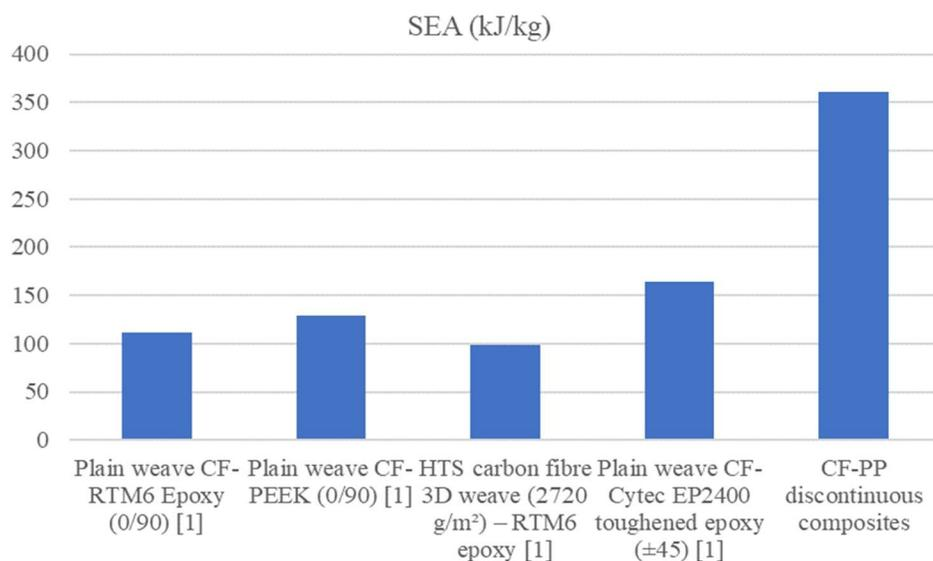
**Figure 1.** Specific energy absorption of the traditional composite materials and discontinuous composites.
