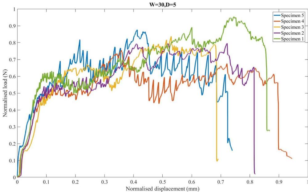
Figure 1: Normalised Load vs displacement of CF-PP discontinuous composites
