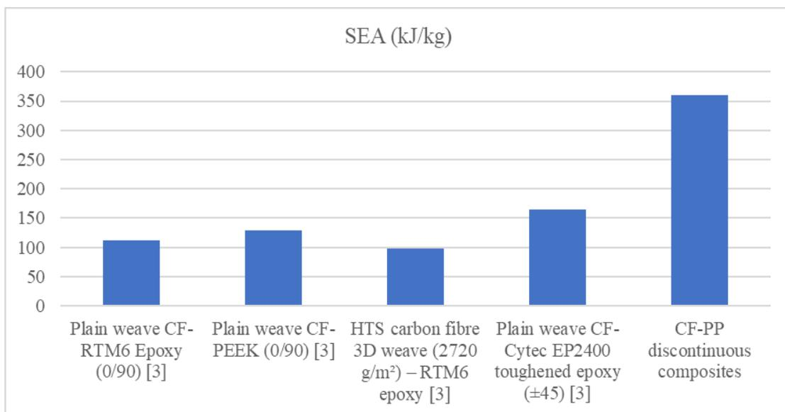
Figure 2: Comparison of SEA of various types of fiber reinforced laminates
