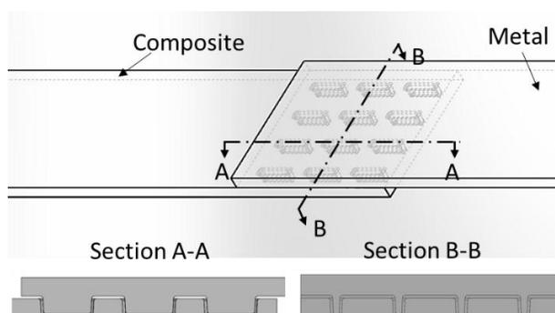
**Figure 1.** Interlocking adhesive joint design
