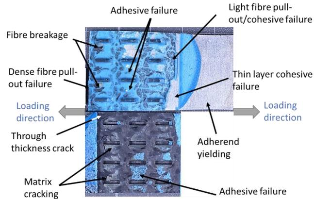
Figure 6: Typical failure surface of IAJ tested at 0.5m/s test velocity
