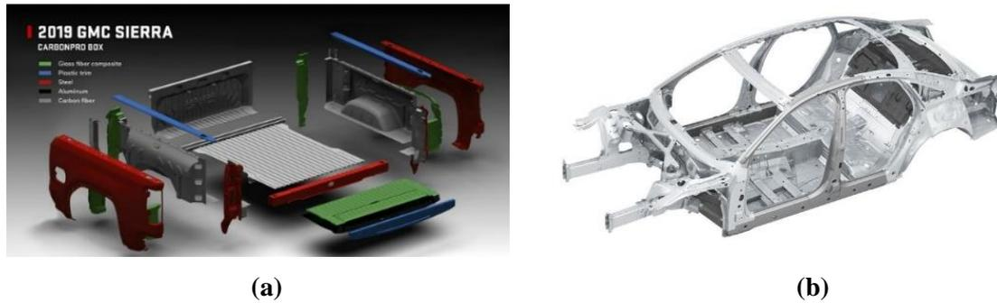
Figure 1. Automotive structures employing multi-material construction: a) GMC Sierra – the truck bed, b) Audi A8 – space frame [1]
