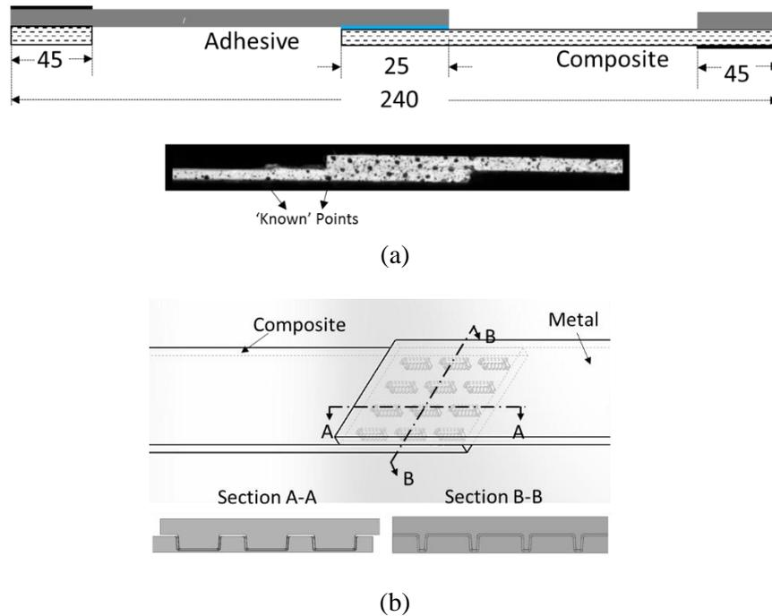
Figure 3: Single lap joint and Interlocking adhesive joint specimens (a) specimen geometry and 'speckled' surface for image analyses (b) schematic of interlocking adhesive joint
