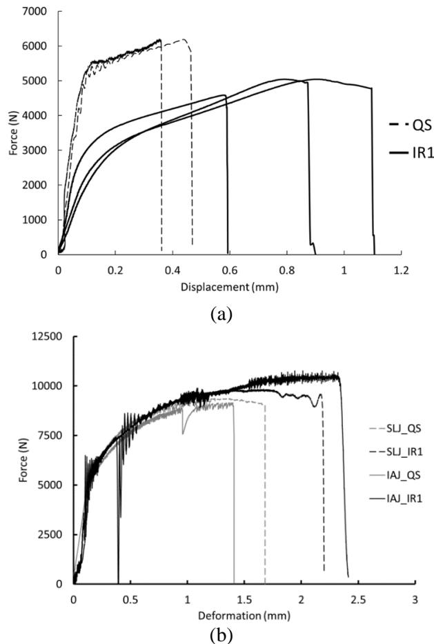
Figure 4: Force-deformation characteristics (a) SLJs bonded with ductile acrylic adhesive (b) Representative curves for SLJs and IAJs bonded with epoxy adhesive tested at QS and IR loading rates
