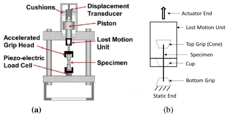
Figure 2. High-speed servo-hydraulic test system: a) schematic of Zwick Amsler HTM 5020 [10] b) lost motion cage
