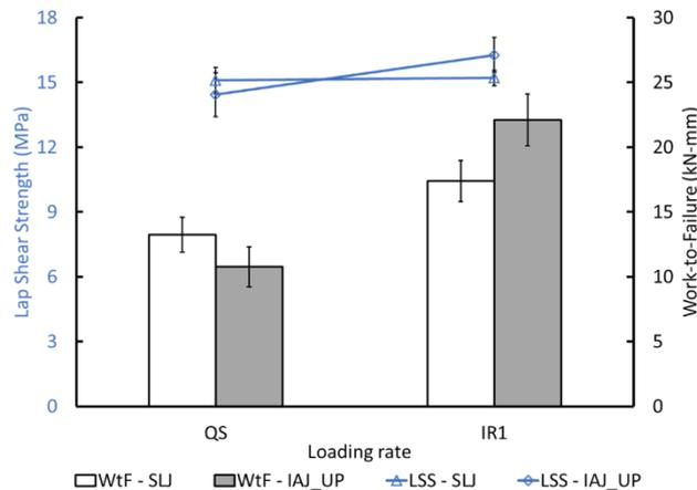
Figure 5: SLJ and IAJ performance characteristics at quasi-static and 0.5m/s loading velocities.
