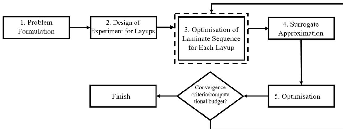
**Figure 1.** Optimisation algorithm for layup and laminate stacking sequence
