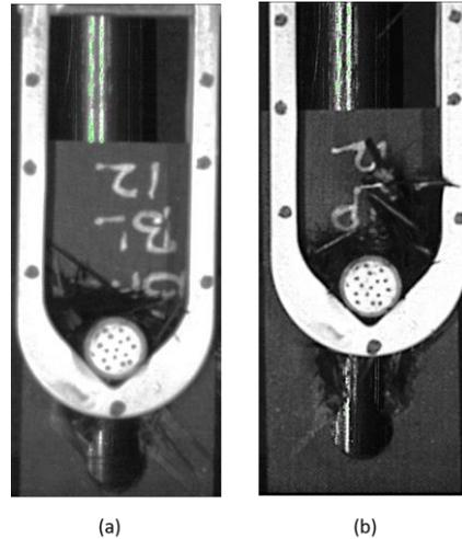
Figure 5: Failure of “Layup 3” specimens with  $D = 12$  mm, (a) blocked and (b) interspersed
