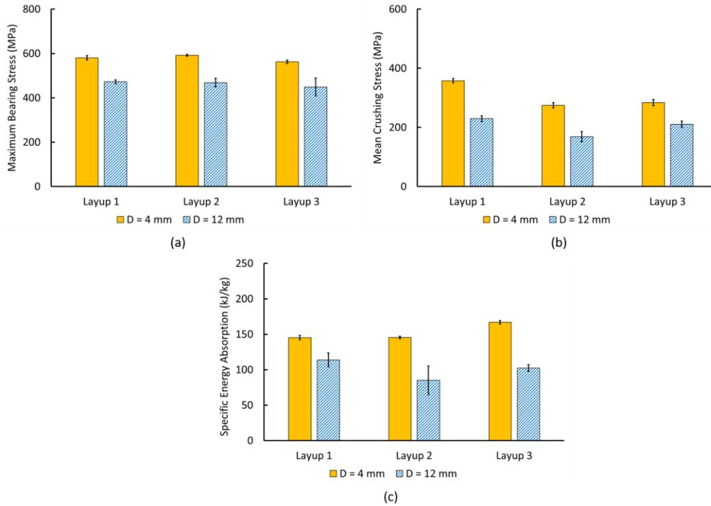
Figure 8: Effect of pin diameter on (a) Maximum bearing stress, (b) mean crushing stress and (c) energy absorption for interspersed ply layups
