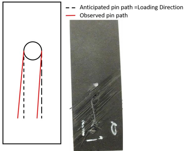
Figure 3: Pin off-axis movement and surface ply peeling in interspersed ply stacking of “Layup 1”
