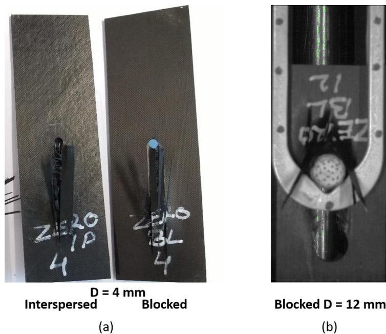
Figure 4: (a) Failure behaviour of “Layup 2” specimens tested with  $D = 4$  mm for both interspersed and blocked ply grouping and (b) specimen tested with  $D = 12$  mm for blocked ply grouping
