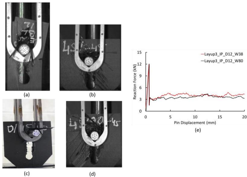
Figure 6: (a) Net-tension failure observed in narrow specimen. Wider specimen tested with  $D = 12$  mm for (b) Layup 1, (c) Layup 2, (d) Layup 3, (e) force-displacement response for specimens with different widths having interspersed Layup 3
