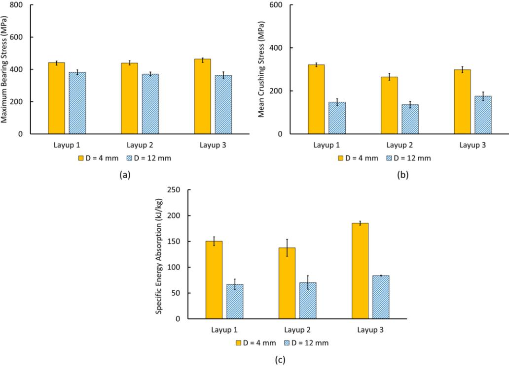
Figure 7: Effect of pin diameter on (a) maximum bearing stress, (b) mean crushing stress and (c) energy absorption for blocked ply layups
