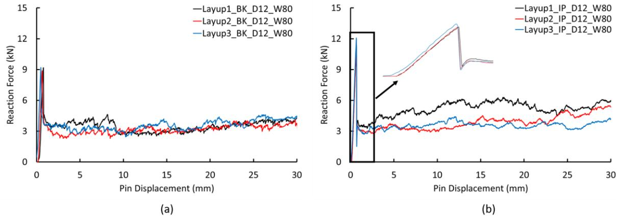
Figure 2: Force-displacement response for different layup specimen of thickness 2 mm, width 80 mm and tested with pin diameter 12 mm for plies grouping (a) blocked and (b) interspersed
