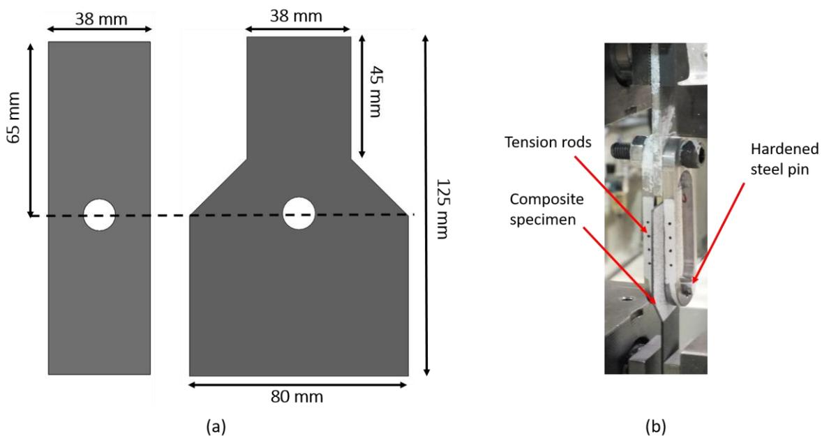
Figure 1: (a) Geometries investigated (b) Test setup
