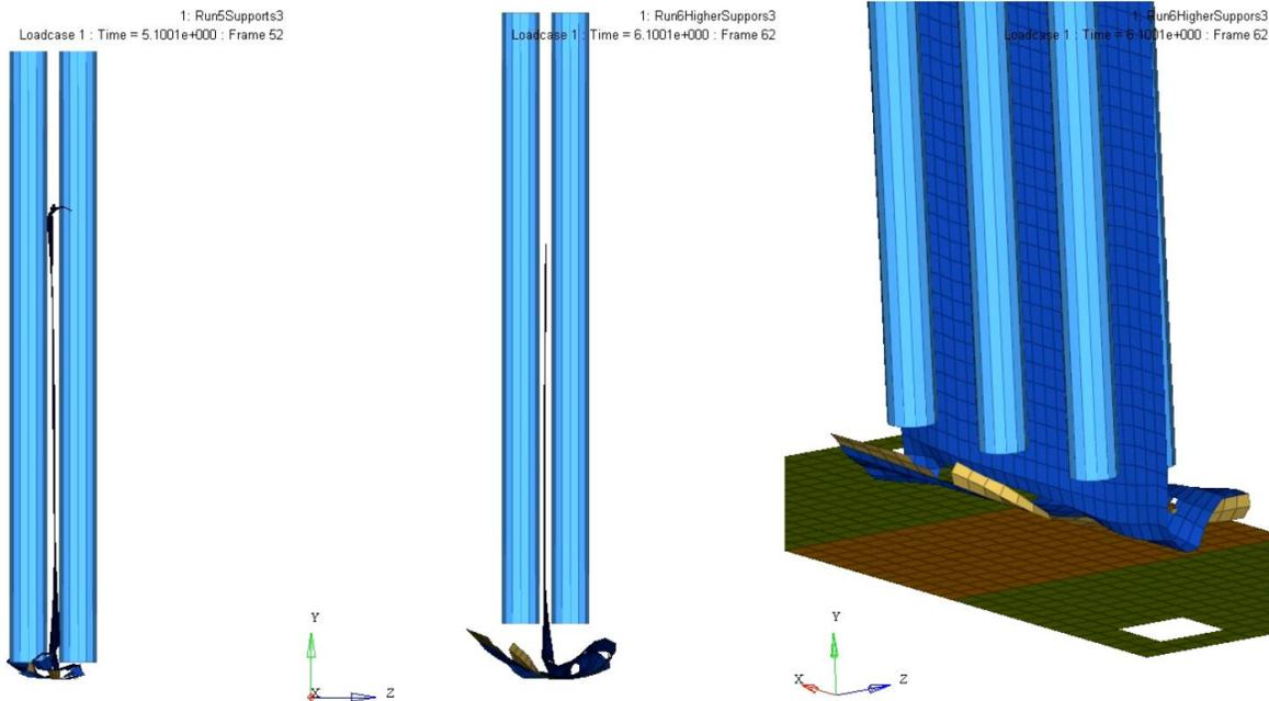
**Figure 2.** Preliminary results of effect of different unsupported heights on flat specimen crushing. Increase in unsupported height from 10 mm to 20 mm causes the specimen to not crumple up, and instead to form fronds as would be expected under impact.
