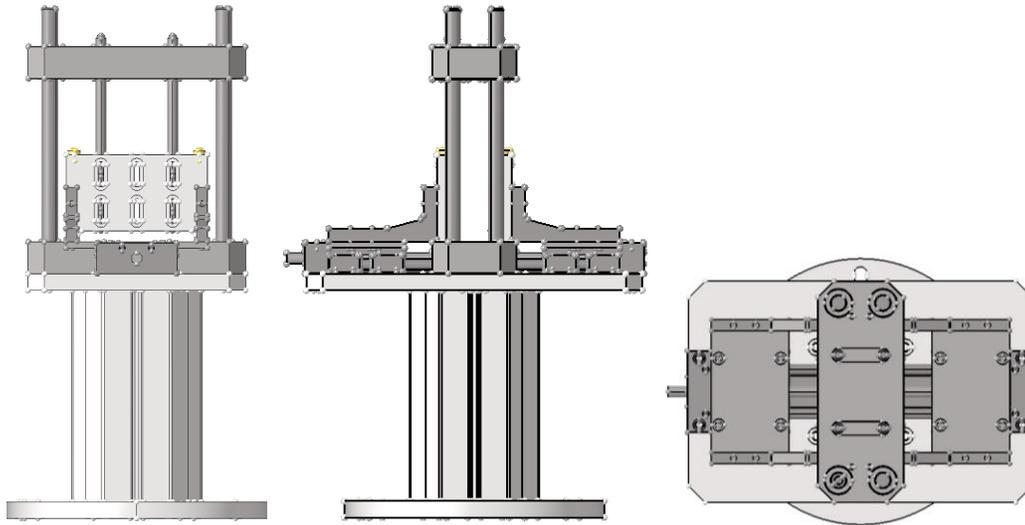
**Figure 1.** Fixture for flat and curved composite testing (Left: Front view, Centre: Side View, Right: Top View).
