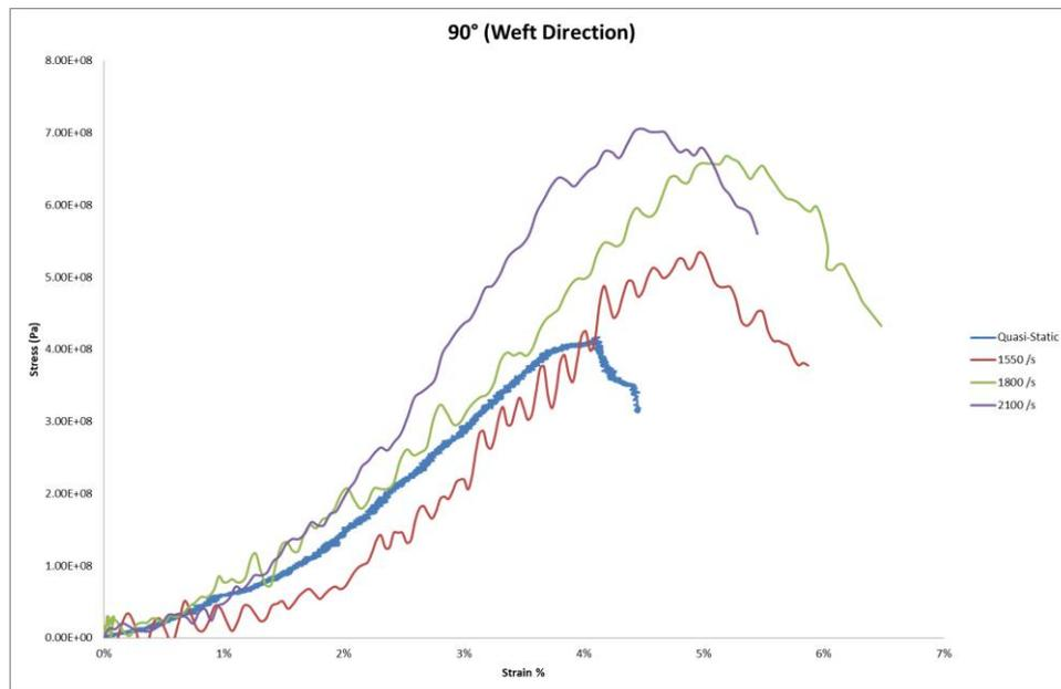
Figure 9. Stress–Strain responses of satin weave carbon/epoxy laminate for weft loading
