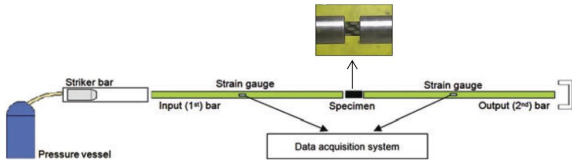
Figure 3. Schematic diagram of SHPB setup
