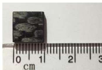
Figure 2. Compression Specimen
