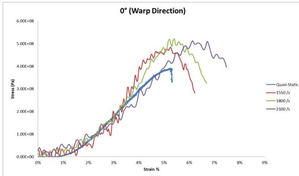
Figure 7. Stress–Strain responses of satin weave carbon/epoxy laminate for warp loading
