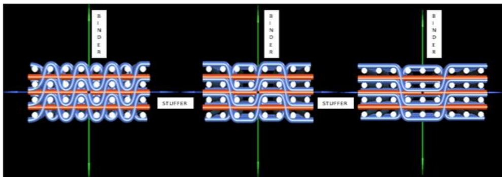
**Figure 1:** Diagram representing three different float lengths in the 3D woven layer-to-layer architecture
