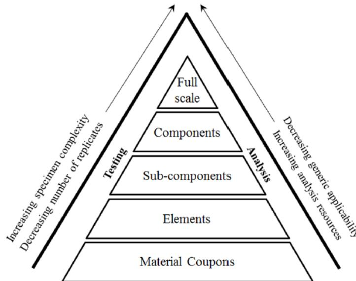
**Figure 1.** Building Block Approach for composite structural development. [2]
