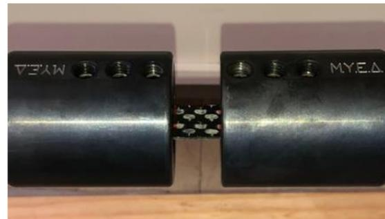
**Figure 1.** (Left) SHPB with high speed camera facility at the University of Patras. (Right) SHPB Tensile Fixture
